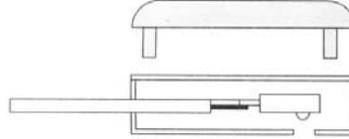
FIG. 3 REMOVING THE FACTORY-INSTALLED SHELL
