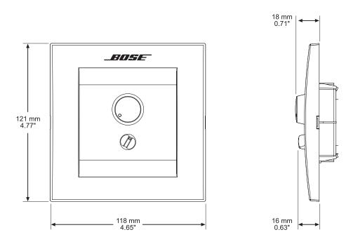
**Note:** The Bose<sup>®</sup> Volume Control User Interface is the same dimensions as the Volume Control with A/B Select User Interface shown above.
