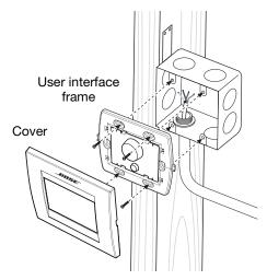
After securing the user interface frame to the junction box, snap the cover onto the frame. To remove the cover, insert the flat head of a screwdriver into the slot on either side of the cover.
