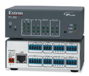
The IPL 250 is an Ethernet control processor that is designed to work with an Extron TouchLink™ panel to create a configurable touchpanel control system. It combines a high performance Web server with three bidirectional serial ports, four IR ports, four relays, and four contact closure inputs for interfacing with common A/V devices and room systems.
